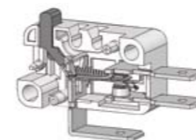
Application of contact profile as a switching contact used for a micro switch.
